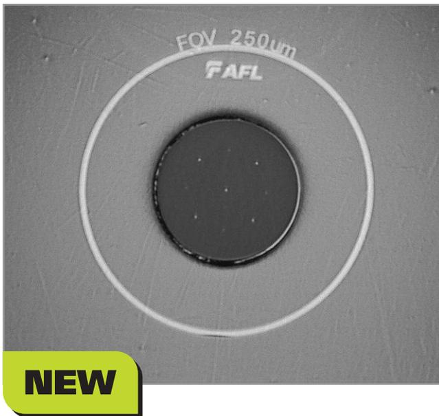
AFL SimpleView Fiber Inspection Software is an application that permits the NOYES DFS1 Digital FiberScope to be used with Windows® XP or Windows® 7 computers. AFL SimpleView software provides a live, high-resolution video image of the end-face of an optical fiber. This capability enables fiber installers and network technicians to inspect and troubleshoot optical fibers and verify that they are clean and undamaged.
